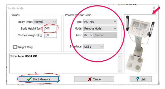
Make sure that your TANITA device is switched ON (and is on PC-mode), that the cable is inserted in the device and in the computer and then press 'Start Measure' to initiate a measurement.
